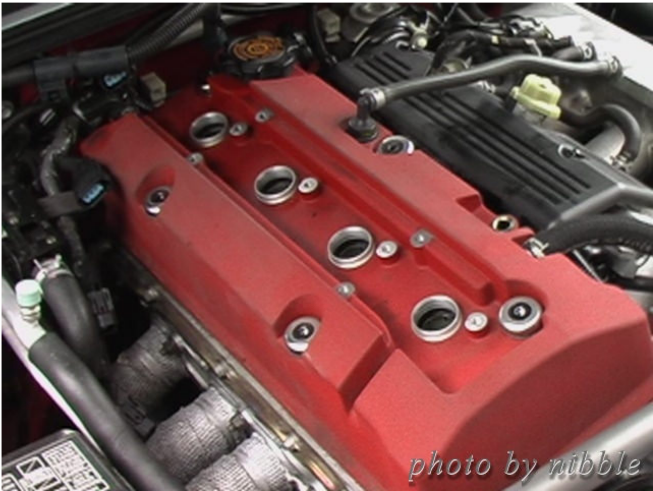
Bill's trick : lift all spark plug connectors first about an inch then remove harness.
