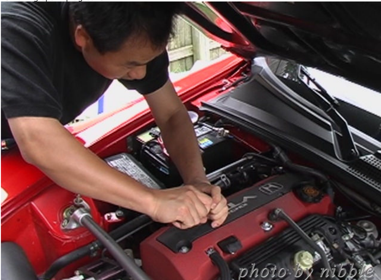
removing spark plug cover.
