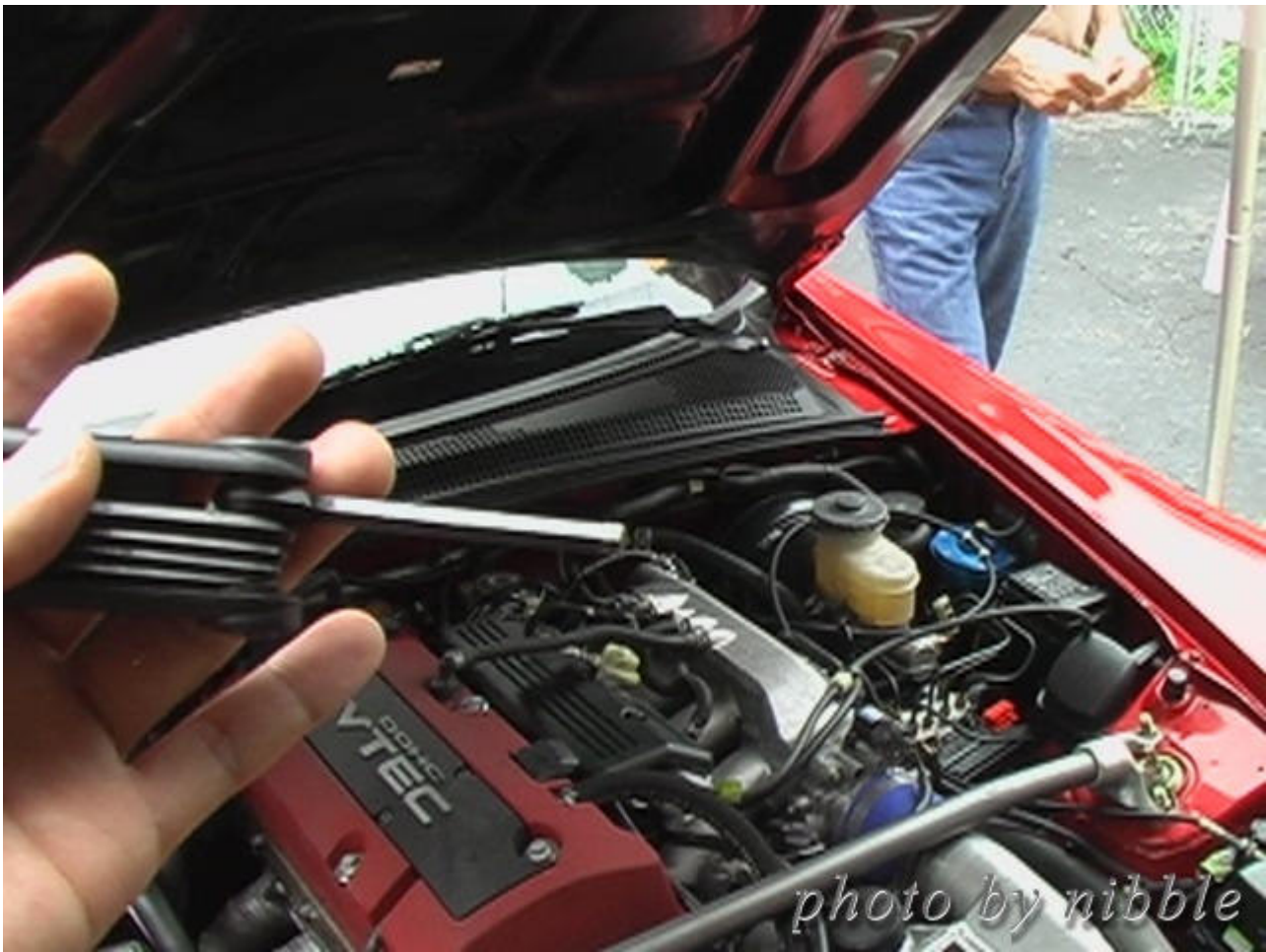
removing spark plug cover.
